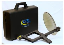
of the dish allow a user to detect ultrasound emissions from a significantly greater distance than when the UL101 is used alone. A co-axially mounted, trigger-activated laser pointer augments indication of the PowerBeam 300's aim point.
